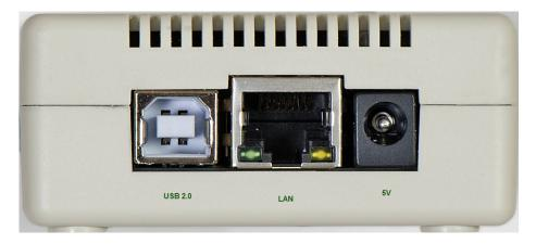
Version with a latching 5V power plug (in production beginning 2019)
