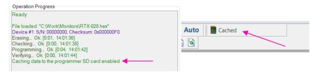
Now we need to generate the serial number information for writing serial numbers into target devices. To do this, either click on the caching status field or select menu **Configure -> Data Caching...:**
