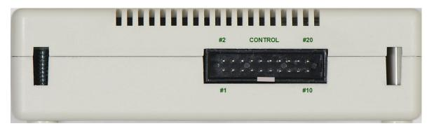
On the picture above a polarization notch of the male connector is situated on the bottom edge of the connector. To control a CPI2-B1 device programmer from your test fixture or other ATE use the
