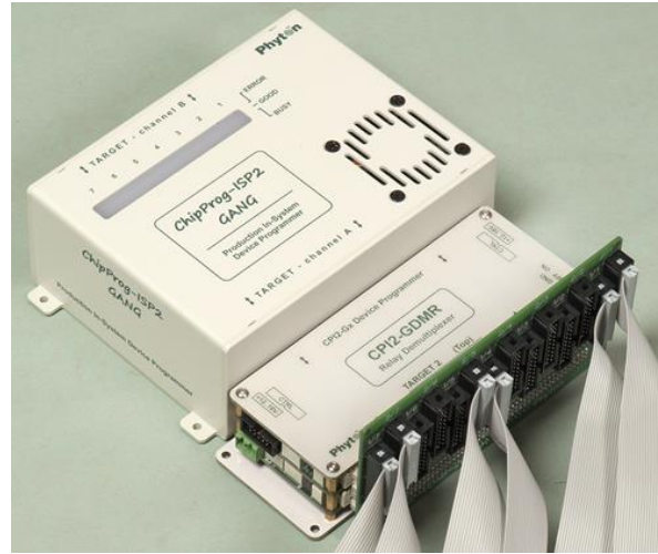
A splitter board connected to the CPI2-B1 demultiplexed channel A through a CPI2-GDMR relay demultiplexer
