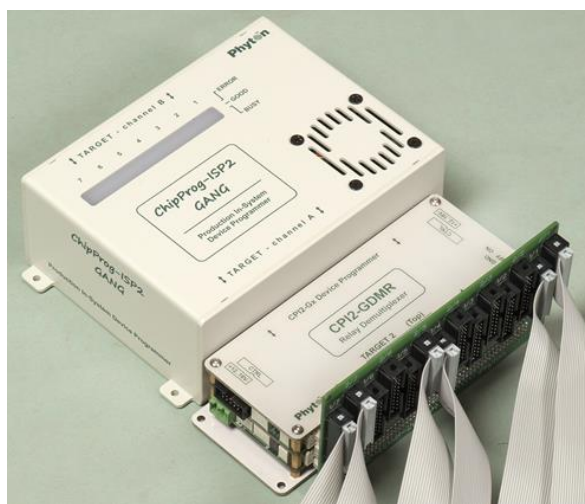
A splitter board connected to the CPI2-Gx demultiplexed channel A through a CPI2-GDMR relay demultiplexer
